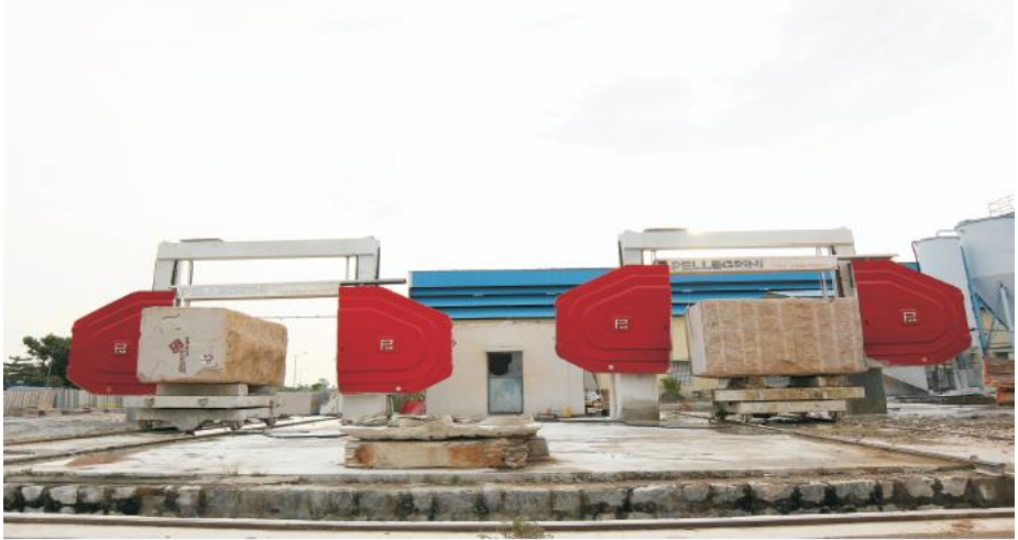
Granite wire saw cutting at TAMIN Granites Plant, Melur, Madurai District.
